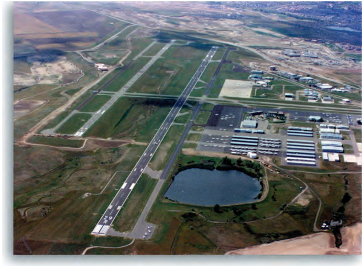
Aerial View of an Airport Showing Runways, Taxiways and the Ramp Area
