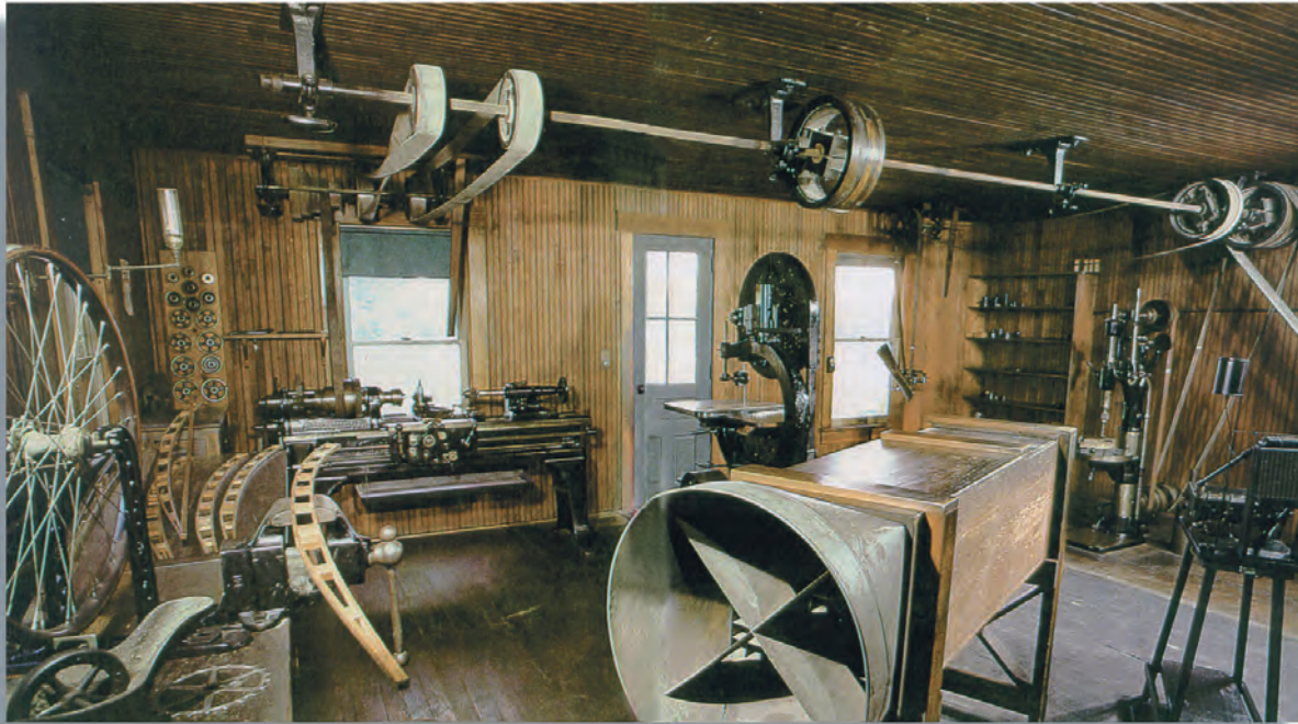
This is the Wright brothers' workshop at Dayton, Ohio, which was reconstructed at the Henry Ford Museum in Dearborn, Michigan. Their wind tunnel stands between an aircraft engine (far right) and a workbench cluttered with wing ribs. The overhead shaft was turned by an engine that the brothers built. It also ran the shop machinery.
