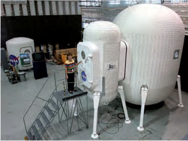
NASA refers to this as the planetary surface habitat and airlock unit.
