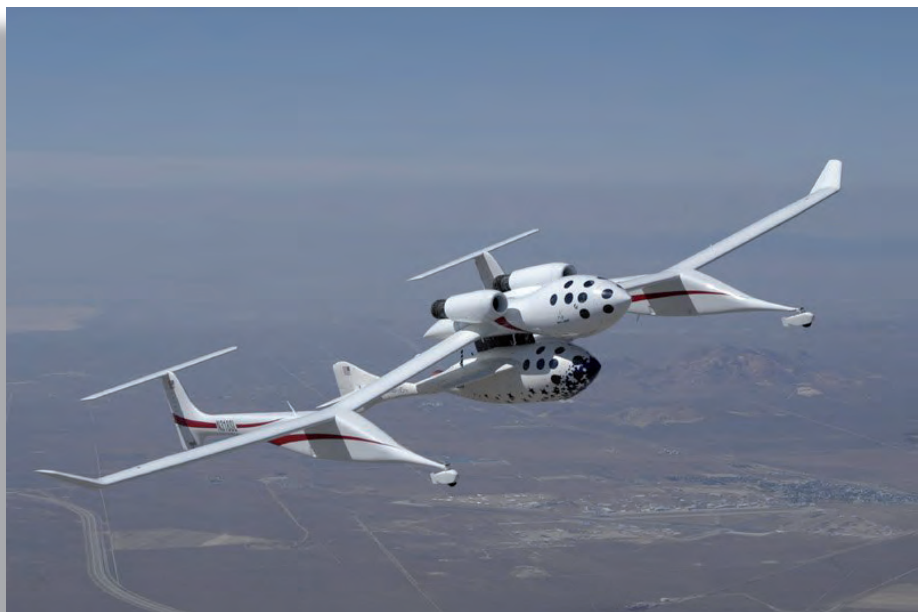
The White Knight "mother ship," SpaceShipOne is released at 50,000 and the White Knight then returns to the airport. (Permission granted to Civil Air Patrol by Mojave Aerospace Ventures LLC, photo by Scaled Composites. SpaceShipOne is a Paul G. Allen Project.)
