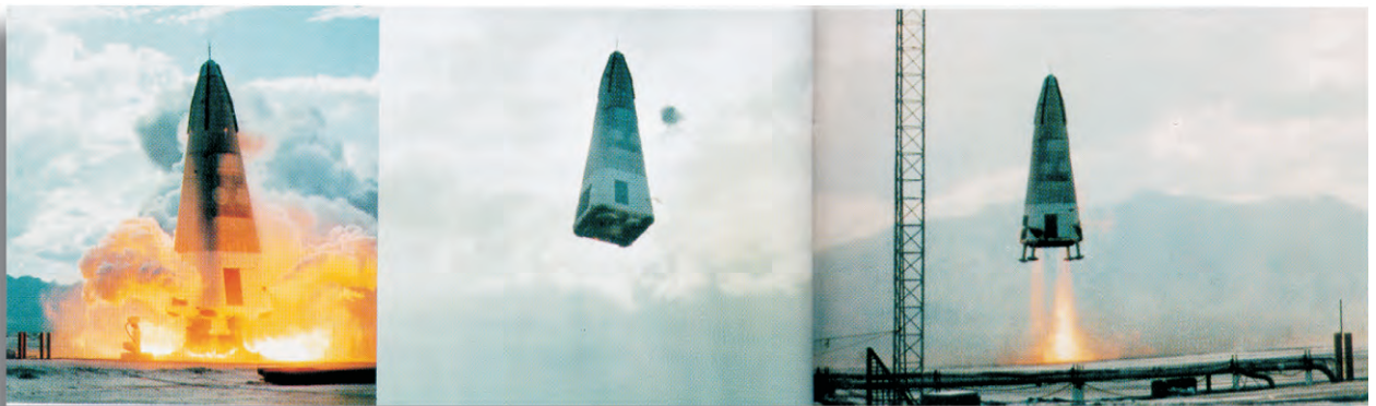
The Experimental DC-X Delta Clipper takesoff and lands vertically, and will be a breakthrough in low-earth orbit.
