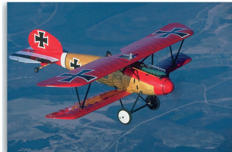
The German Albatros D-II had a plywood fuselage and two machine guns. (EAA)
