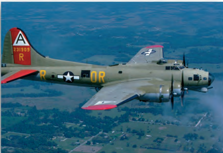
An American B-17 Flying Fortress. Note the guns in the nose, rear, sides and on top. (EAA)
