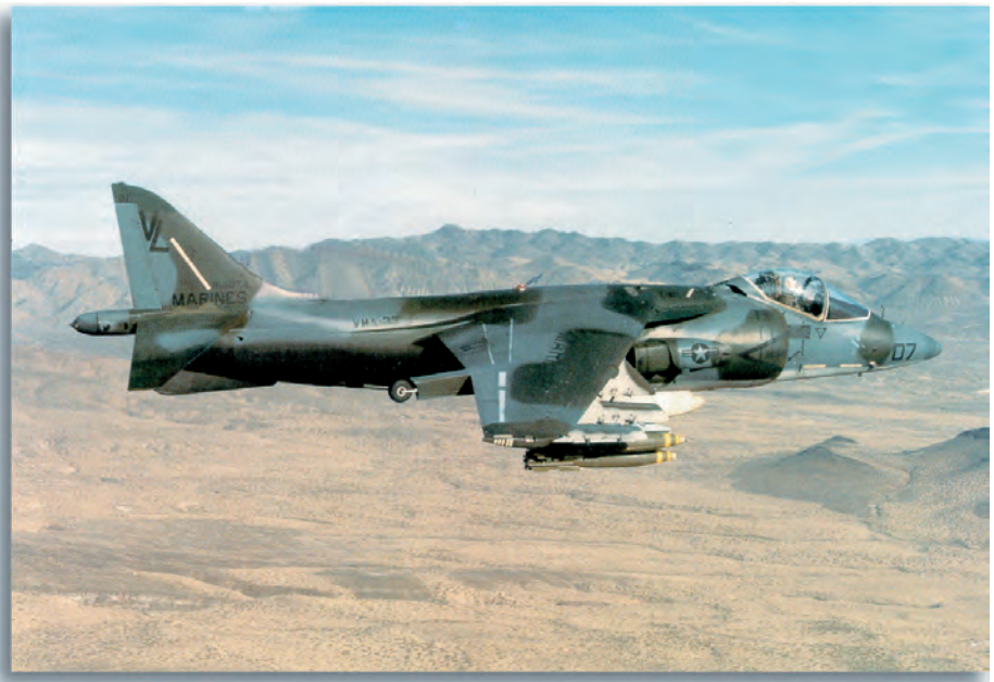
The McDonnell Douglas AV-6B Harrier II was originally developed by the British and is currently in use by the US Marine Corps. It can hover like a helicopter, yet fly an attack mission at speeds in excess of 500 mph.
