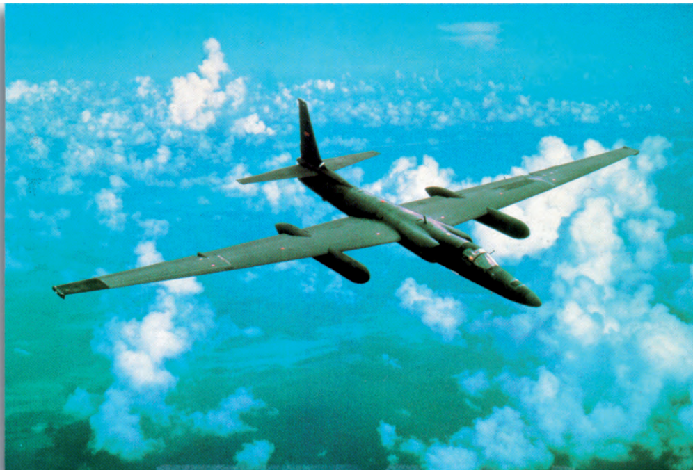
The Lockheed TR-1A spy plane could operate at altitudes well above 90,000 feet.
