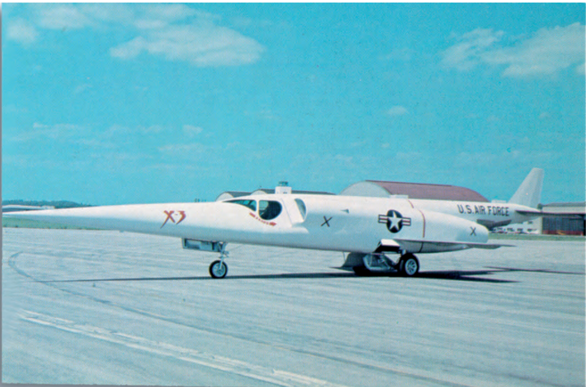
The Douglas X-3 Stiletto was designed for aerodynamics, structural and other flight research in the Mach 2 range.
