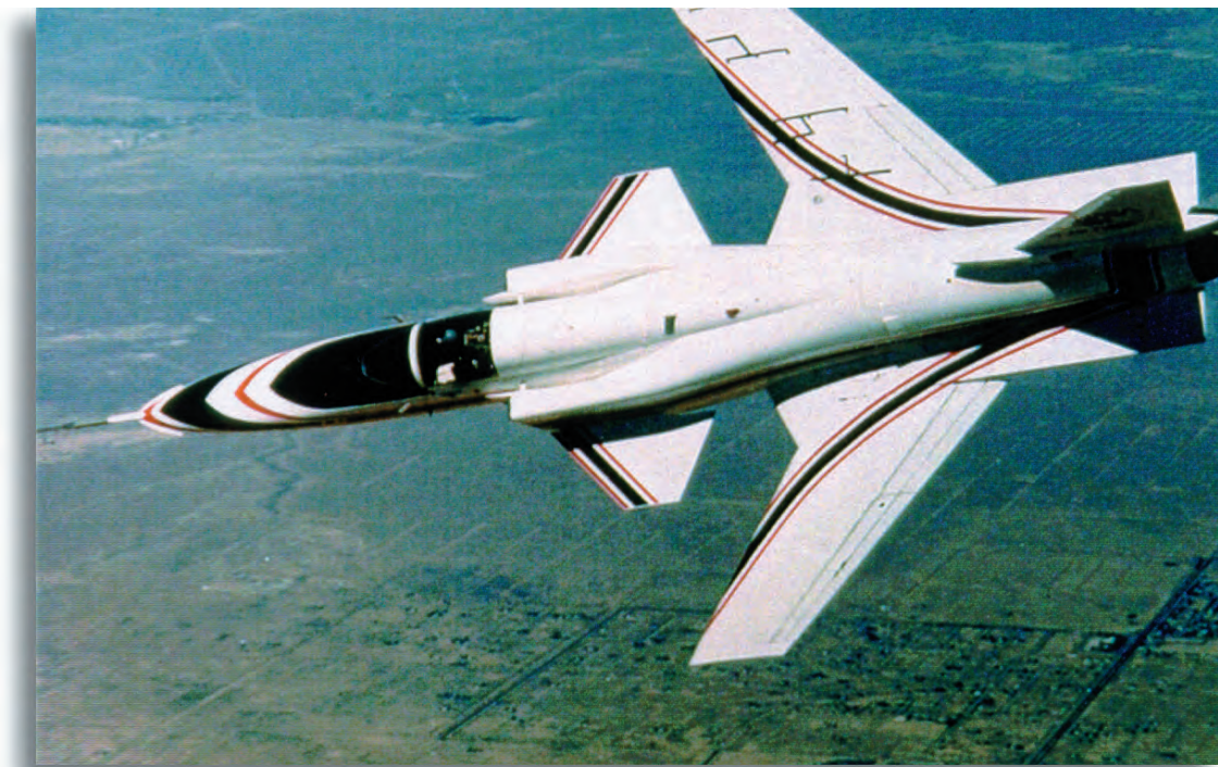
The forward-swept wings of the X-29A
