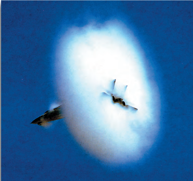
A ring of condensation occurs in the wave as this F-14 goes supersonic. (US Navy)
