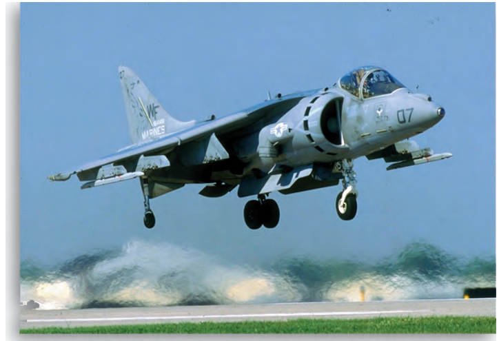
The AV-8 Harrier has a tandem landing gear. (EAA)
