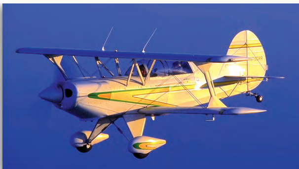
The Aerosport II has fixed landing gear. (EAA)
