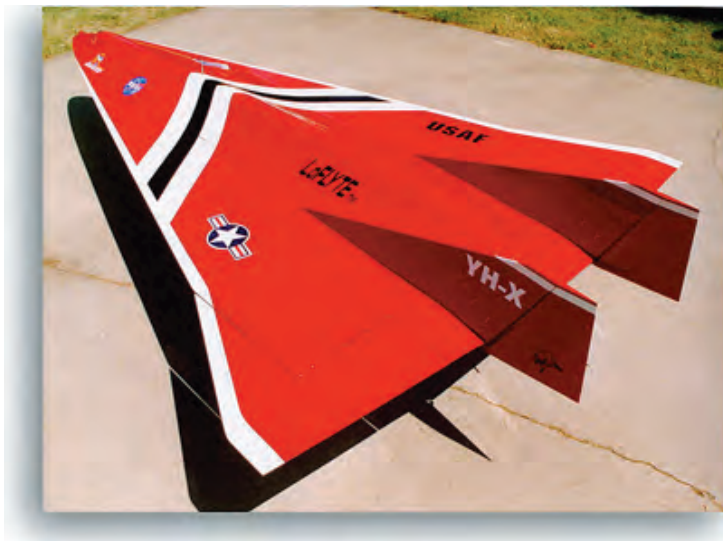
LOFLYTE (Low-observable Flight Test Experiment) is used to explore new flight control techniques involving neural networks, which allow the aircraft control system to learn by mimicking the pilot.
