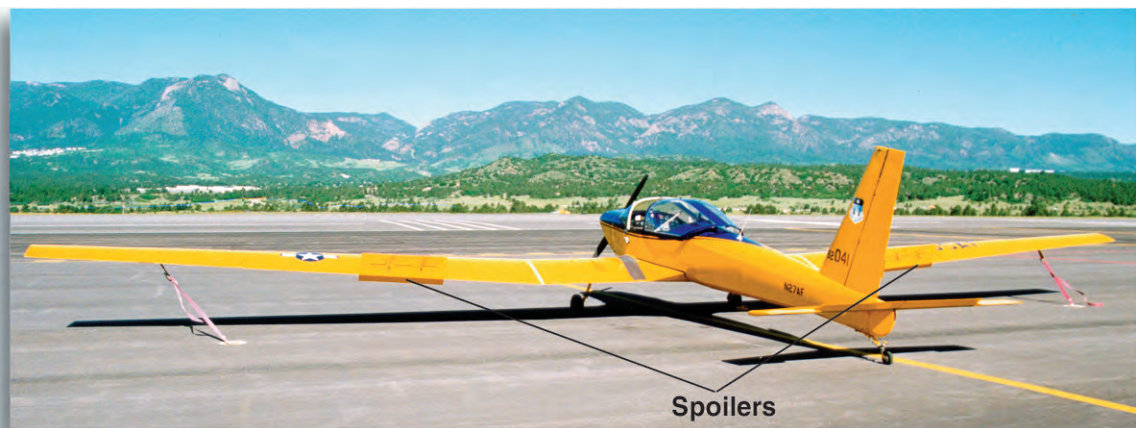
This Air Force Academy TG-7A has spoilers above and below the wing. They are located just inboard of the USAF insignia.
