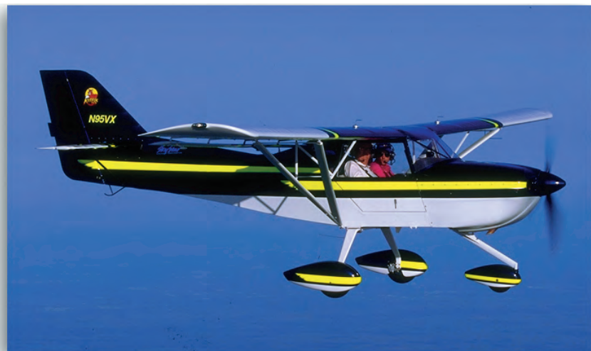
This is an example of tricycle landing gear. (EAA)
