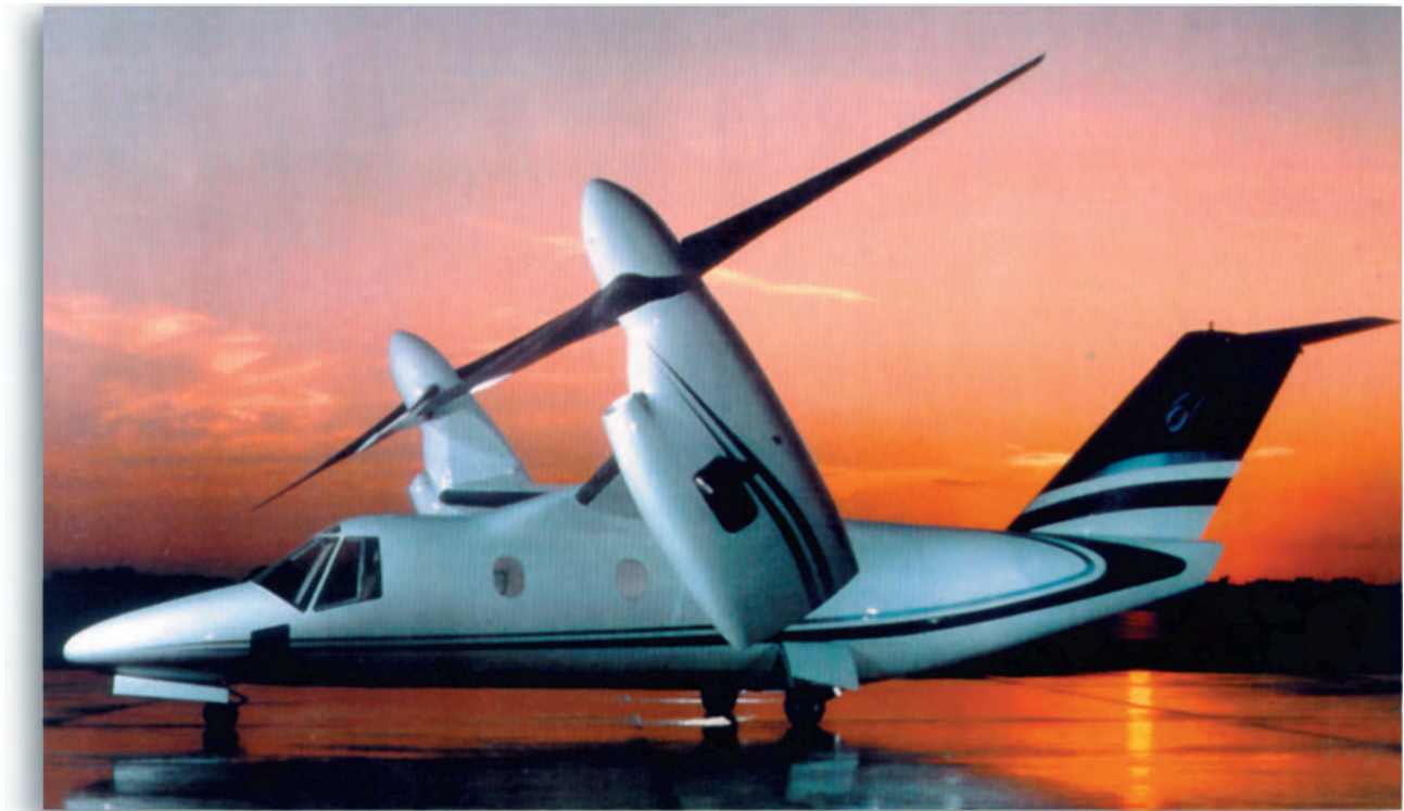
The Bell/Augusta 609 is a commercial tiltrotor aircraft. (Bell Helicopter Textron Photo)
