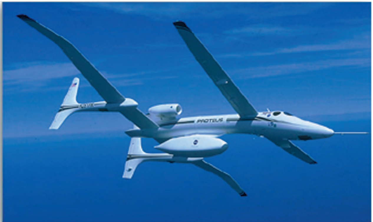
The Proteus , designed by Burt Rutan, has a front-mounted airfoil called a “canard.” It provides lift and pitch control. (EAA)
