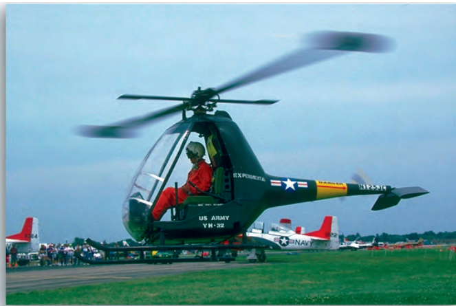
In the early 1950s, a ramjet (on the blade tips) was used to power an experimental helicopter known as the Hiller Hornet . (EAA)
